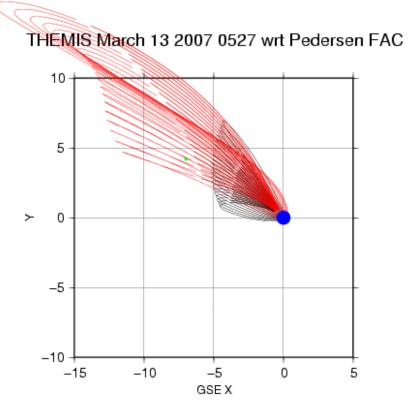
The Pedersen FAC of the ARM model can be mapped to space with GEOPACK (Courtesy N. Tsyganenko and GSFC). THEMIS A (green) is between the FAC sheets. One could model the FAC flowing along these field lines.
