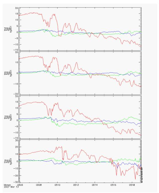
Radial and/or westward propagation of disturbance near 05:08 onset using field-aligned magnetic perturbations. X (blu) is toward Earth, Z (red) is along the field and Y (grn) westward.
