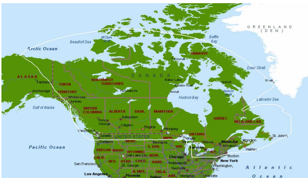
Figure 5: Anik F2 satellite footprint (white outline) showing coverage of Ka-band high speed satellite internet service.
